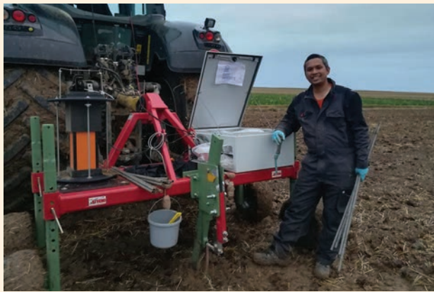
Fig. 2 Experiment done by using a passive gamma-ray spectrometer and visible NIR spectrophotometer to measure the micronutrients in soil
